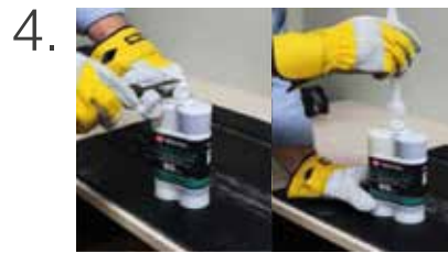
Remove the buckle and fasten the mixing tip
