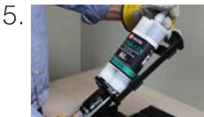
Place the cartridge in the spray gun
