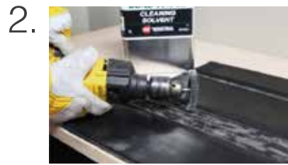
Roughen the working surface
